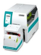
The **THERMOMARK E.WRAP** applicator automatically applies labels to wires between 2 and 16 mm in diameter (14-6 AWG) while ensuring consistent wrap and placement on the wire. The device has an adjustable scale, so the label is always applied at the desired distance from the wire end. Self-laminating wire wrap labels are an extremely resilient identification solution that can even be used in outdoor applications.
